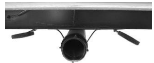
Black/Grey Tank Drain and Valves
